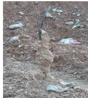
> 图9 普通抗浮锚杆成桩外观 > Fig.9 Appearance of common anti floating anchor
