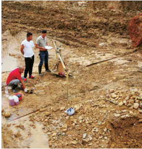
> 图11 普通抗浮锚杆基本试验 > Fig.11 Basic experiment of common anti floating anchor
