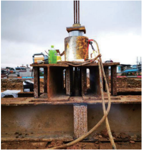
> 图12 复合锚杆基本试验 > Fig.12 Basic experiment of composite anchor
